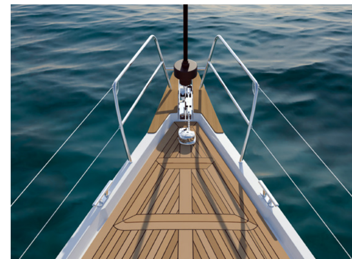
In the foredeck a deep sail locker, with integrated self draining anchor chain compartment. The electric anchor winch capstan can be fitted with an optional topwinch to operate moorings.
