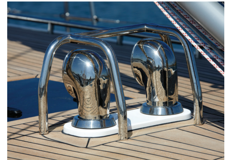
Stainless steel ventilation dorades are mounted on the coach roof, with stainless steel protection bar, provide excellent ventilation into the accommodation.
